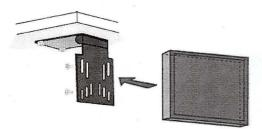
Fit the bracket to the back of the LCD screen with the bolts supplied.
